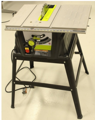
Figure 29. Bench Saw Modified by ES Staff
