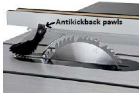
Figure 4. Typical anti-kickback pawls.
